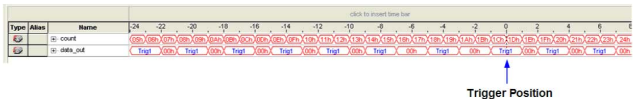
Figure 92. Signal Tap Logic Analyzer Continuous Data Capture
