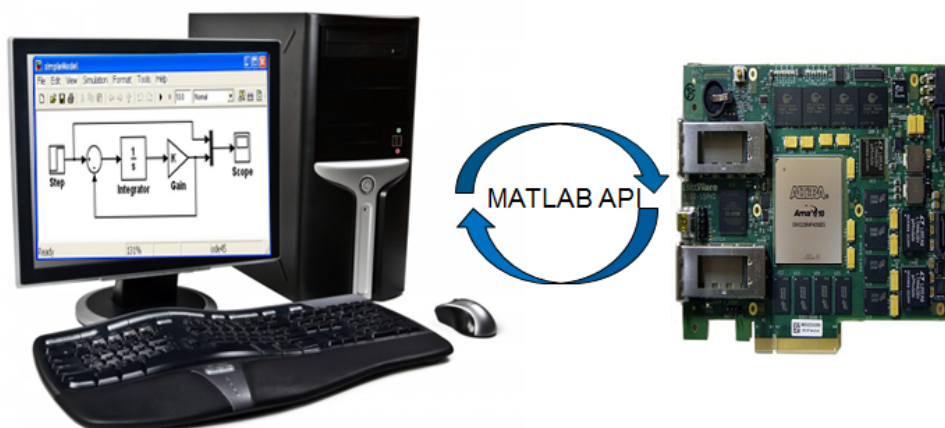
Figure 128. Hardware in the Loop Host-Target Setup
